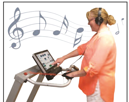
The Gait Trainer 3 provides real-time biofeedback and quantifiably displays step length, step speed (spm) and step symmetry.
